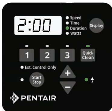
Figure 12: Setting Duration for Quick Clean
