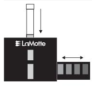
The Octa-Slide Viewer should be held so non-direct light enters through the back of the comparator. With sample tube inserted at top, slide the Octa-Slide bar through the viewer and match with color standard.
