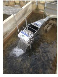
Manual use, a tank is connected to the fish counter inlet, a water pump provide water flow through the counter
