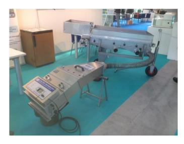
Fish counter connected to the fish grader
