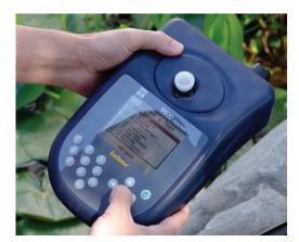
Parameters: Alkalinity Aluminum Ammonia **Bromine** Hardness Chloride Chlorine Chromium Color Copper **Cyanuric Acid Dissolved Oxygen** Fluoride Hydrazine Hydrogen Peroxide Iron Magnesium Manganese Molybdate Nickel Nitrate Nitrite Organophosphonate Ozone pН PHMB Phenol **Phosphate** Potassium Silica Sulfate Sulfide Sulfite Zinc
