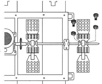
After proper attachment of the outer paddles there will be about 6 inches of the axle sticking out (notch numbers 7 and 8 are not used). It is not necessary to remove the extra length of axle.
