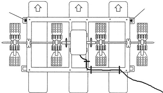
Under normal operation the paddle wheel exerts such a force back toward the shoreline it is necessary to tie or stake it down in place. Stakes are provided with each paddle wheel. They should be placed through the metal loops on the water outflow side of the frame.
