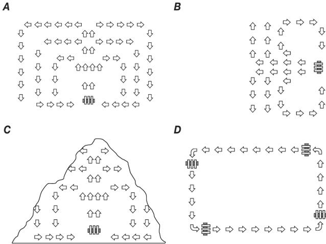
In hill ponds (watershed ponds) paddle wheel aerators are most efficient when placed at the middle of a dam (Figure C). In larger, rectangular ponds of many acres, several paddle wheels are often placed to create a circular flow pattern (Figure D).
