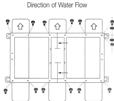
On each long side of the frame, measure from the outer edge of the frame to the first hole encountered on the center crossbars. On one side the hole will be approximately 10" from the edge, and on the other side the hole will be approximately 12" from the edge. The short side (10") should be on the same end as the water flow as indicated by the pontoons.
