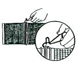
Lock all three parts together by inserting the snap-fastener(s) as shown.
