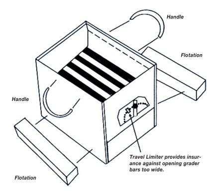
To assemble, align floats and handles with existing holes on the main body of the grader, thread the bolts through and tighten.
