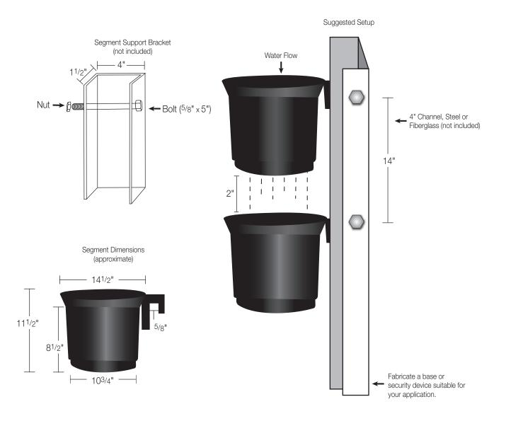
Enclosed you will find one (1) retaining disc for each aeration bucket ordered. Once the disc is securely placed in the bottom of each segment, add packing media. Support bracket (part no. **AB12A**) sold separately.
