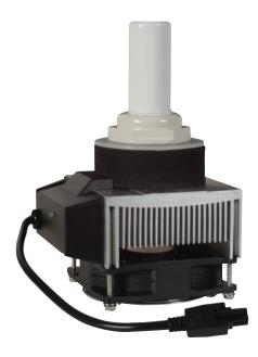
The Coolworks Ice Probe®, uses advanced thermoelectric technology to directly convert electricity into cooling power. A unique, patented design, based upon Peltier's Principle, makes it a highly efficient miniature heat pump.
