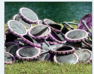
All diffusers need maintenance, even ones with rubber membranes.
